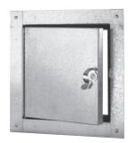
to facilitate cleaning the duct of accumulations of dust and combustible materials. Service openings shall be placed at approximately 20 foot intervals along the duct and at the base of each vertical riser. Service openings shall be sized and shall incorporate access doors coded manufactured by Duro Dyne Corporation.
