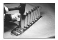
4. Insert the top rail tabs into the vanes.
