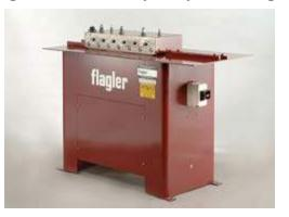
This machine is designed for heavy gauge Pittsburgh locks. Complete with hardened feed gauge, 3 piece roll/shaft/gear construction, and calibrated dial for 18-22 Ga. mild steel.
