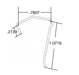
All measurements are inside dimensions Manufactured from 22 Gauge
