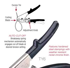
Tensioning Adjustment knob and automatic cut-off mechanism Turn Adjustment knob clockwise to increase tension and counter clockwise to decrease tension. CAUTION: Do not over tighten adjustment knob with fingers. Adjust knob only with fingers to avoid breaking ties before cut-off occurs.
