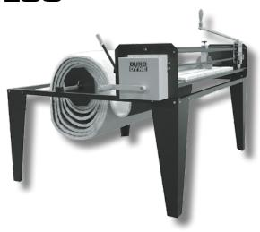
The LSU Advance Liner Sizer will help size and cut duct liner more efficiently than ever thought possible with a hand operated machine. It's enhanced features, make it possible to cut cotton fiber insulations, filter media, rubberized products and other unusual materials. The cross cut and slitter blades are mechanically gear driven to spin while cutting. This spinning action shears the material to create precise cuts in the most difficult of substances.
