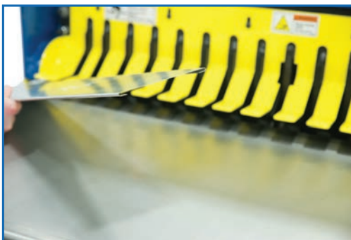
Open-end design allows L-Shaped ducts to be formed
