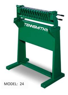
TENNSMITH's cleat benders are manually operated tools that form uniform drive cleat edges on rectangular ductwork in seconds without set-up or adjustment. The upper handle forms the cleat and the lower handle opens the tool for easy removal of the material. Heavy cast iron and fabricated steel construction provides long life and trouble-free operation. A TENNSMITH cleat bender can save you time and money.
