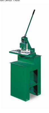
The TENNSMITH notcher, Model 16-18, is a versatile, heavy-duty bench tool for shearing, notching and piercing work. The heavy cast iron construction allows the notcher to be used to side shear six inches of material to its rated capacity; and the throat behind the upper ram is beveled on one side to permit long strips of material to pass without restriction.
