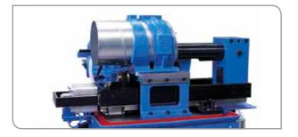
The new generation of SPIRO® FLYING SLITTER, utilizing extra strong linear guides in combination with the strength of the toggle joint, results in the perfect cut.
