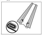
Bend seam up to 90° on brake as indicated in drawing.
