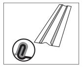
Using heavy snips, notch standing seam at bend points.
