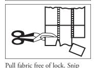
severed lock as indicated. Ends of metal are now ready for Option B: bending and joining.
