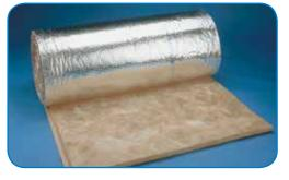
**Composition and Materials:** SoftTouch Duct Wrap is a blanket-type insulation composed of tan, uniformly textured, inorganic fibrous glass formed with a formaldehyde-free, plant-based binding agent. It is available unfaced or with FSK, gray PSK or white PSK vapor retarder facing. On faced products, a stapling/taping tab is provided on one edge.
