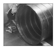
Complete the gasket application by installing Ductmate Neoprene gasket on the face of the flange around the entire circumference of one of the mating flanges.
