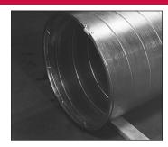
5. The break in the flange will allow a portion of the leading edge of the duct to be visible. Apply a short piece of Ductmate 440 gasket to the flange face over this visible leading edge on **both** mating flanges.\*
