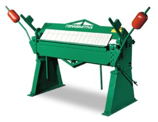
This brake features a removable apron insert for 1/4-inch bends in lighter material. The upper leaf adjustment screws feature thrust bearings to prevent upper beam creep. Ductile steel clamp handles, heavy counterweights and an apron stop rod add to the brake's ease of operation.
