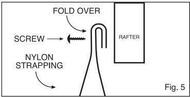
FOR A NICE ROUND BEND, INSTALL THE DUCT SADDLE SLING APPROXIMATELY 18" AWAY FROM THE PRE-INSULATED BOX.
