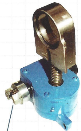
Heavy duty worm gear screw jack arrangement for positioning bending rolls. Alloy steel guide block holds SKF sealed spherical roller bearings.
