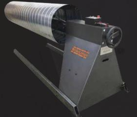
The **SideLiner** consists of 110 volt, 15 amp, reversible variable speed control with E-stop and spindle lock, and wireless remote start/stop function.
