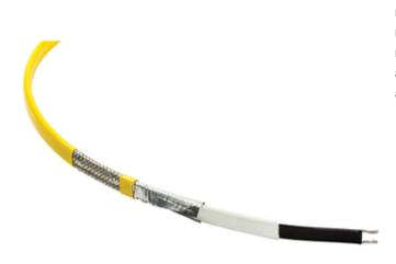
nVent RAYCHEM HWAT self-regulating trace heating cables maintain water temperatures in a building's hot water distribution network. Installed underneath the thermal insulation, they automatically compensate for pipe heat losses where they occur and provide an energy efficient solution.
