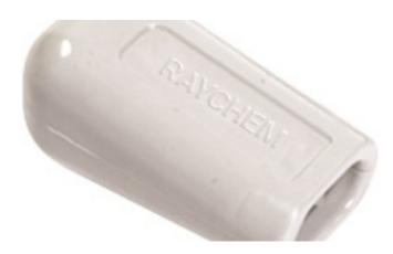
nVent RAYCHEM RayClic-E-XX end seals are a simple, fast and reliable end termination developed for select nVent RAYCHEM XL-Trace, IceStop and HWAT self-regulating heating cables. No heat guns or wire stripping are needed, because silicone gel technology is used to make the electrical termination.
