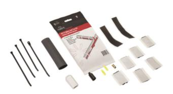
RAYCHEM WinterGard H910 Splice and Tee Kit is for use with WinterGard self-regulating heating cables to make splice, tee, and end seal connections. The kit contains materials for one splice and one end seal, or one tee connection and one end seal. This kit does not provide a power connection; use an H900 or H908 power connection kit for a complete installation.
