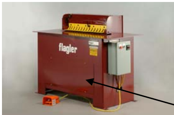
Remove this lower panel to view main motor.
