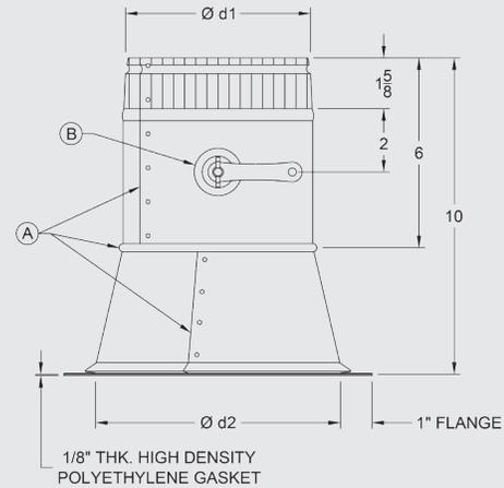
A. Conicals now come standard with sealed joints! The riveted seam on the collar and cone, as well as the co-latch seam between the collar and cone are sealed with the GreenSeam integral gasket. Unsealed fittings are available upon request.
