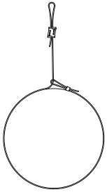
No Ferrule Around Duct
