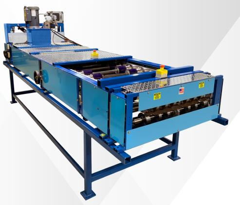
Although originally an agricultural panel, the 5V crimp is now a popular residential panel. Mount the 5V machine in your shop or make it portable and take it to the jobsite. The 5V machine features a hydraulic drive and front hydraulic scissors shear, adjustable panel width capability 14" to 28". The "traditional size" 5V Panel is feeding the machine 27 1/2" coil stock, giving you a 26" wide finished panel with 24" coverage with the overlap.
