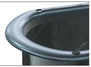
5. Seal the joint internally with PROseal\* duct sealant. Brush the sealer into the joint and onto both the face and inside edge of the connector pieces to achieve a 100% seal.
