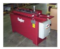
Rollform your drive turn hems on this machine after notching and prior to bending into L or full wrap sections. Simple select the sections to be hemmed with the selector switch and run through. The machine will hem the 1st and 3rd quadrants or the 2nd and 4th quadrants.
