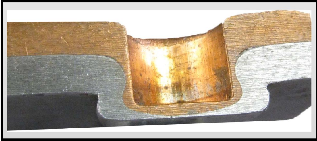
Figure 15 – Cross Section of Joint
