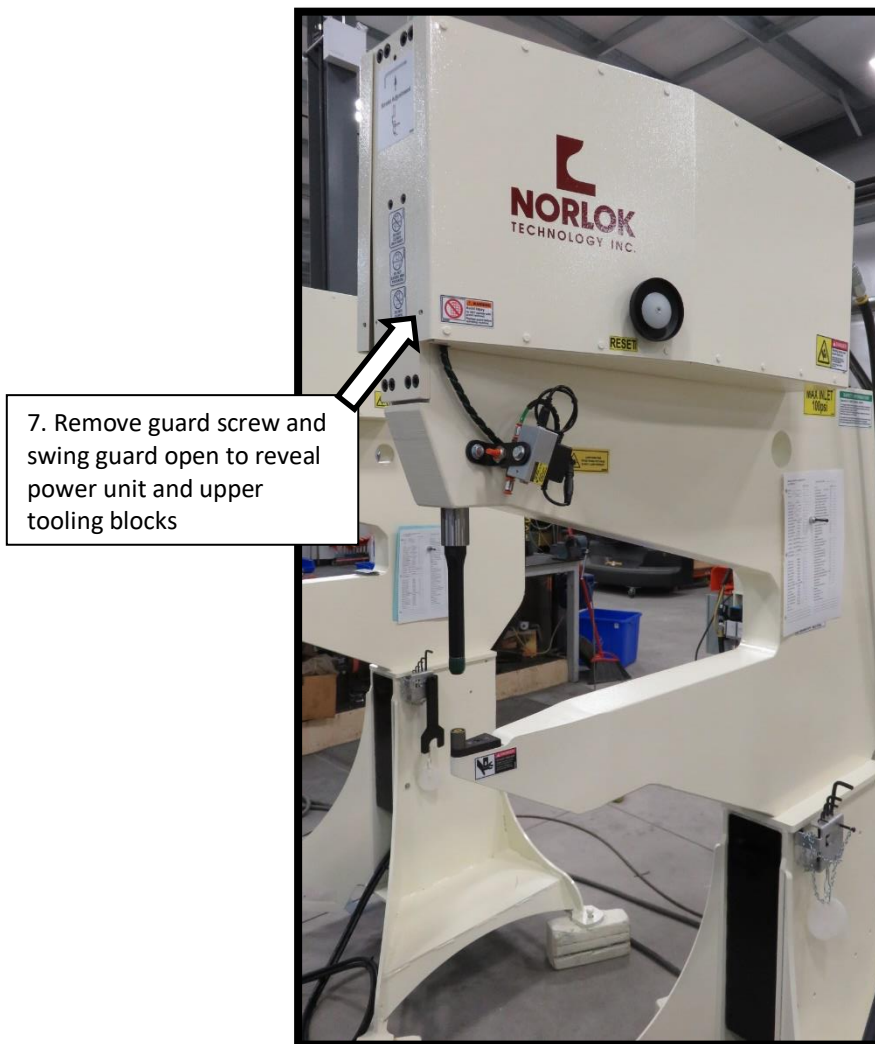
Figure 6 Removing Tooling Guard
