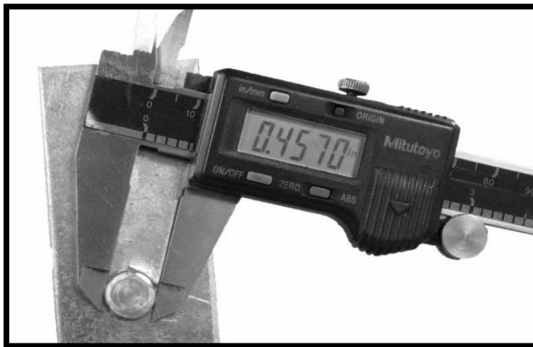
Figure 2 Measuring a Button Diameter (BD) using Vernier calipers
