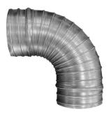
Low pressure and friction loss. Meets SMACNA gauge requirements. Airtight 4-ply lock seam construction. Meets leakage Class 3 for 10" W.G. Duct construction class in a sample test section. Sealant is required only where elbows attach to the duct, saving labor time. Greater structural integrity. 26 ga Galvanized Steel
