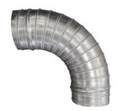
Low pressure and friction loss. Meets SMACNA gauge requirements. Airtight 4-ply lock seam construction. Meets leakage Class 3 for 10" W.G. Duct construction class in a sample test section. Sealant is required only where elbows attach to the duct, saving labor time. Greater structural integrity. 26 ga Galvanized Steel
