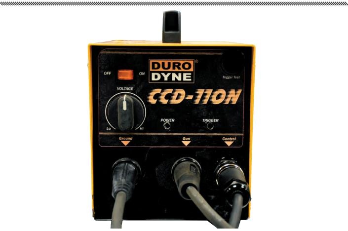
**POWER SWITCH:** The POWER switch applies AC voltage to the power supply Hi/Lo causing the weld capacitors to charge to a voltage level determined by the setting of the VOLTAGE CONTROL. Also, the charge time is dependent on the setting of the VOLTAGE CONTROL, ranging from 1 to 3 seconds.
