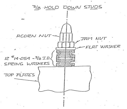
WHEN INSTALLING TIGHTEN JAM NUT
