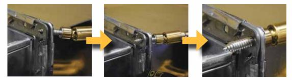
Self-piloting screw tip of the bolt self-aligns the corners and ductwork, eliminating the need for an alignment tool and clamping. 1-1/2" bolt shown.
