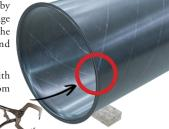
Complete the gasket application by installing Ductmate Neoprene gasket on the face of the flange around the entire circumference of one of the mating flanges.
