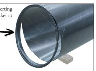
5. The break in the flange will allow a portion of the leading edge of the duct to be visible. Apply a short piece of Ductmate 440 gasket to the flange face over this visible leading edge on **both** mating flanges.\*
