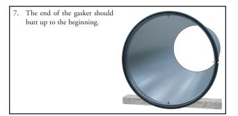
Continue in the same direction around the duct at evenly spaced intervals, as noted below left. Place the last fastener within 1/2" of the end of the duct flange.
