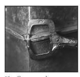
Compress gasket at corners with vice-grip while snapping in corner clips.
