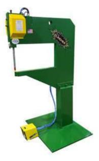
Clinch two (2) pieces of same, dissimilar, or painted metals with 28 to 14 gauge mild steel capacity.
