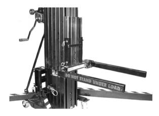
Disengage 4 spring-loaded pins. Rotate fork assembly 180 degrees. Engage the 4 spring-loaded pins.
