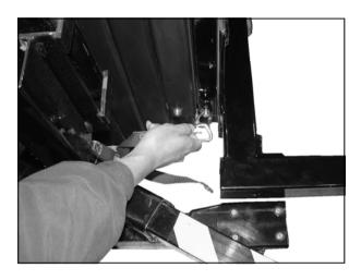
Pull on strap to tighten Hold Down. To remove Hold Down, press lever on cam buckle and slacken Hold Down strap. Remove Hold Down from Safety Latch Loop on side of fork.
