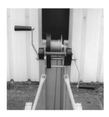
Use the winch to crank forks up or down into the desired position. Then crank winch handles up about 1/4 turn to set the safety brake.
