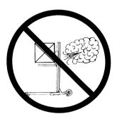
Operate only on level surfaces. Use the unit on smooth and level surfaces to avoid unit tipping over and the possibility of operator injury.
