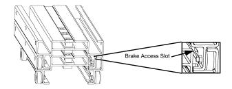
Pull the tool down and the brake will release.
