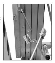
To release Hold Down, pull bar toward you and place back behind mast sections.
