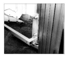
Disengage 4 spring-loaded pins. Rotate fork assembly 180 degrees. Engage 4 spring-loaded pins.
