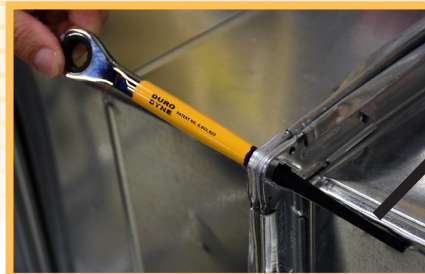
The 9" long drift pin end allows you to align two corners in a flange connection without struggling or clamping
