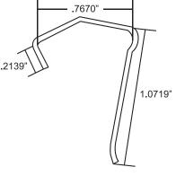
All measurements are inside dimensions. Manufactured from 22 ga.
