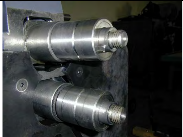
Remove Top and Bottom Rolls from the machine
