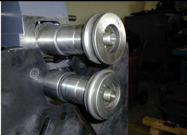
Remove Locking nuts from top and bottom shafts.
