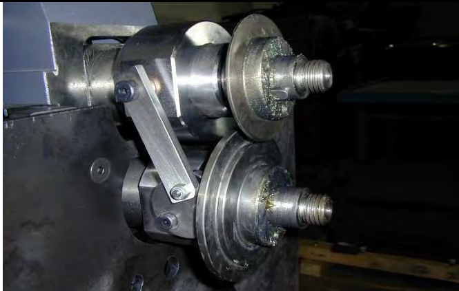
Install the inner bottom roll onto the bottom shaft and then install the inner top roll onto the top shaft.
