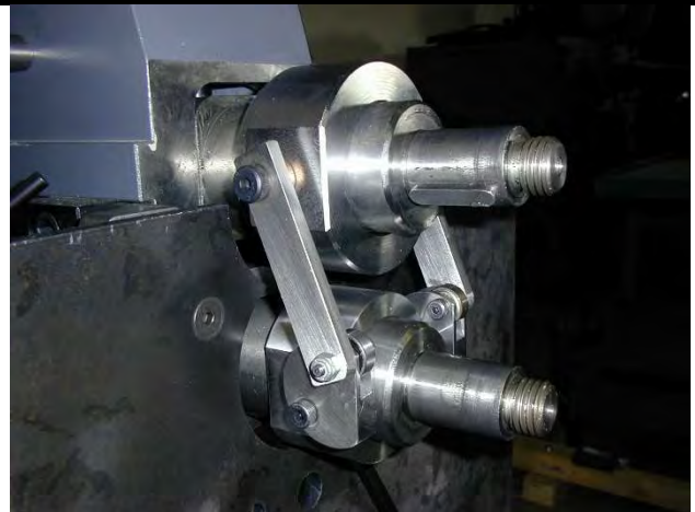
Install the pusher mechanism by sliding the collars over the shafts as far back on the shafts as possible.
