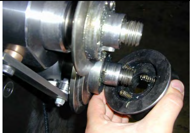
Place the springs in the pockets of the outer bottom roll and align the springs with the pockets on the inner bottom roll. Once springs are in their pockets you can thread on the locking nut to hold the rolls in place. By filling the spring pockets with grease, it makes it easier as the grease keep the springs from falling out.
