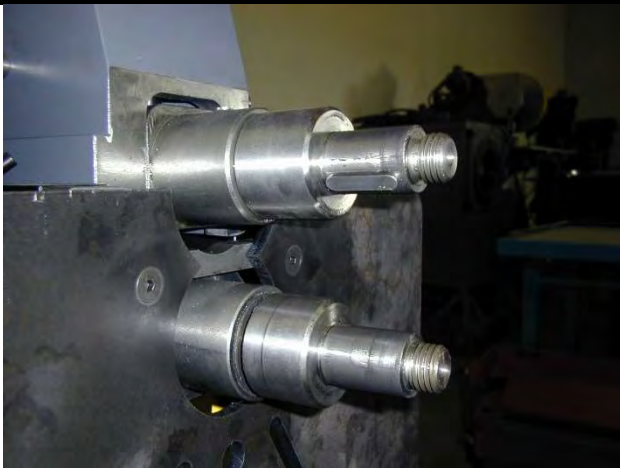
Remove the factory spacing collars from the top and bottom shafts.
